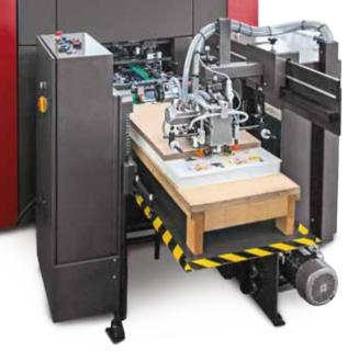
The DCH200 features a **HIGH PILE FEEDER** which will handle a wide variety of stock weights and thicknesses.
